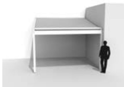
Construction situation 4 - Against a supporting and right-side construction
