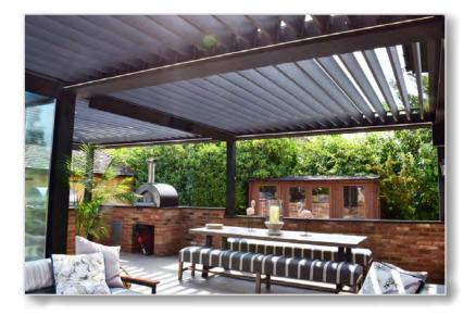
To cover the entire area 3 Renson Camargues would be interlocked for a seamless space, whilst glass sliding walls would create a bright internal environment. We further recommended the inclusion of Rain Sensors within the louvers and automated fix screens at the rear of the space. All of the inclusions can be controlled by remote, ensuring simplicity of control to this sophisticated structure.
