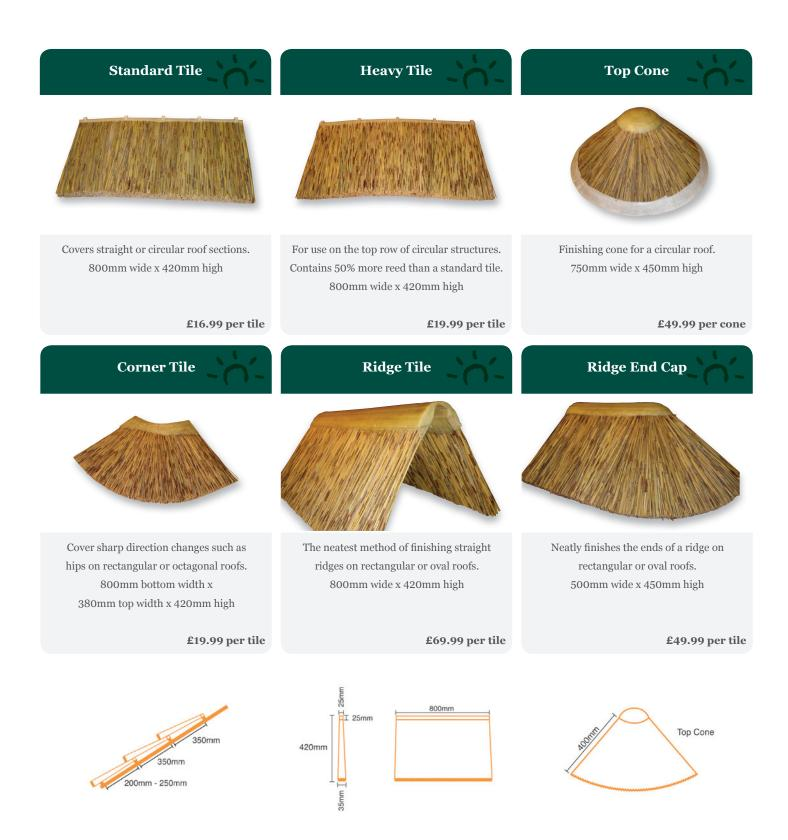
All Cape Reed Thatch Tiles are supplied with attached clips that can be fastened to an 8mm bar or rope and this is the recommended way to install. Alternatively tiles can be nailed to a standard roof batten.
